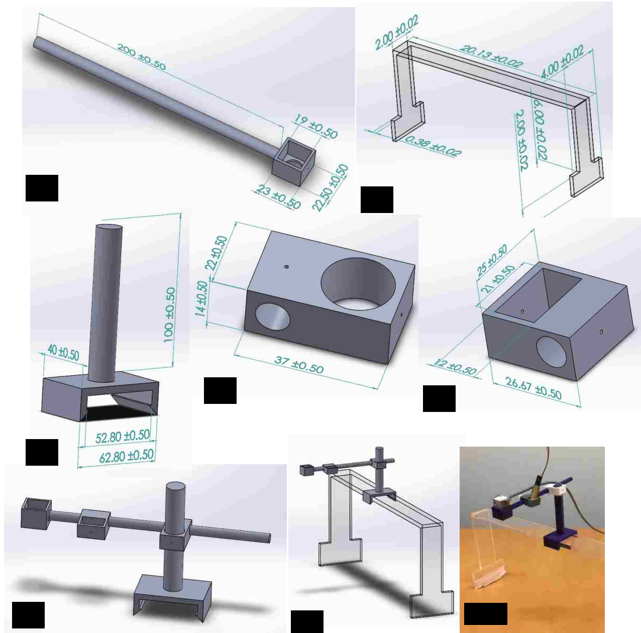
Figure 3.3 Individual pieces of the design and overall assembly: a) camera piece b) plastic bridge c) the base d) base-camera connection e) laser piece f) overall assembly without plastic bridge g) assembly with plastic bridge h) actual assembly looking (with camera and laser)
